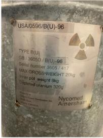
Photos: Type B(U) Package (left) and close up on the label on the type B(U) package (right)
